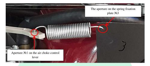
35. Turn the control throttle choke lever on the handbrake switch to the right (in "OFF" position). Install tensioner bolt in throttle choke cable plate  $N_{2}$ . Pass the choke cable through the tensioner cable (1), then through the aperture  $N_{2}$  at the lever (2) and then fix the end of the cable by the  $\emptyset$  3 mm cable fixator (3).
