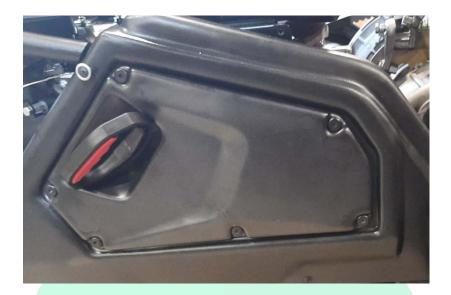
47. Fix left side cap, using screws with inner hex. Set the screw in the central bottom aperture, this screw is shorter than other 10 mm screws because it does not touch the CVT.
