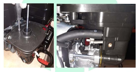
19. Install the two sleeve-nuts from the «Fasteners kit» package №1 on the studs near the manifold.
