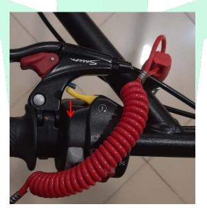
Close the choke- turn the choke control handle to the right. During «cold start», 60 seconds is required. Wait till the engine will get warm and then turn the choke switch off.
