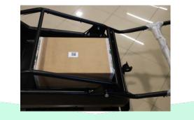
2. Detach bonnet rubber fasteners from the bosses on the frame at the left and right sides. Demount the bonnet.
