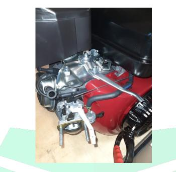
16. Weaken the throttle valve control lever that way, it will easy return back to the original position. Step 25mm aside from lever edge, mark the place of edge you have to saw and saw it off. The final result:
