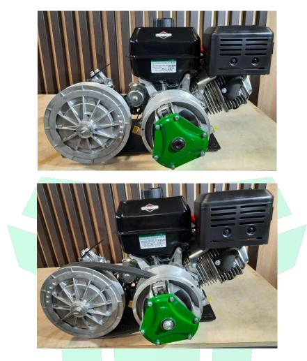
25. Take the CVT belt out of the box and dress it on the CVT. Install the belt on the discs by tightening the belt and rotating the movable disc opposite the clock arrow movement.
