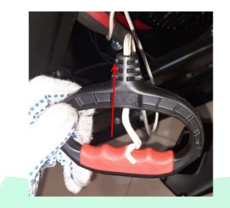
44. Pass the cable through the aperture at the right side cap, and then into the starter handle. Tie the knot and hide it in the handle.
