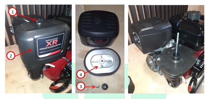
15. Dismantle the air filter fastener (1). Unscrew the manifold fastener nuts (2), twist the bolt out (3) from the rear part of the intake manifold and detach the hose from it (4). Demount the manifold (5).
