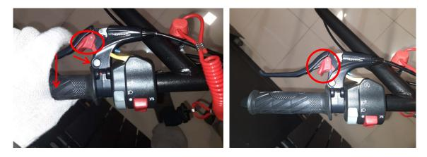
3. Open the throttle valve- turn the control choke handle to the left.
