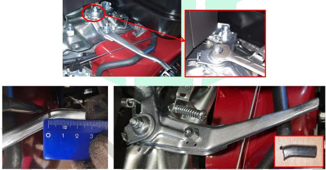
17. Drill the hole in the center at the air choke lever bending. Use the  $\emptyset$  2 mm drill bit.
