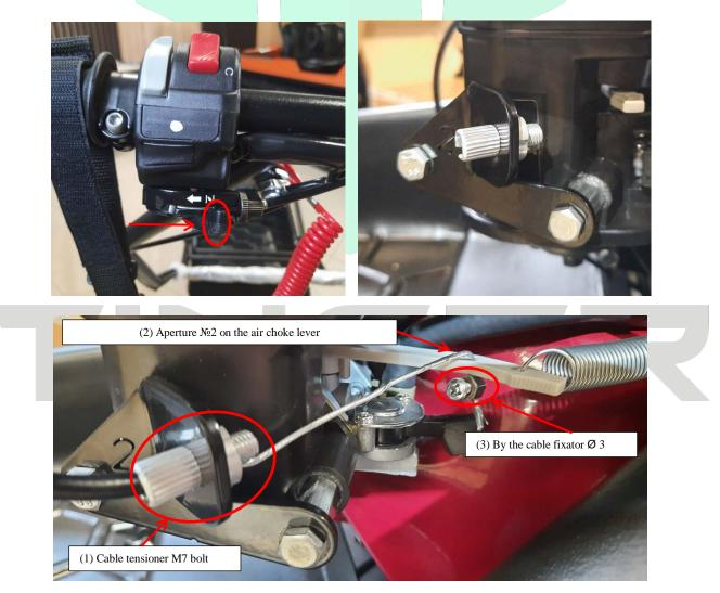
36. Take the Ø 3 mm cable fixator out from the «Springs and retainers kit» package  $N_{26}$ . Spread the brake cable with the red braid's end at the frame along the engine compartment up to the brake
