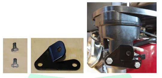
21. Take the spring fastener plate out from the «Spring retainer kit» package  $N_{2}$  3. Unscrew the two top bolts, that are anchoring manual starter cap and weaken the bottom bolt. Install the plate behind the manual starter cap. Look after the left bottom edge of the plate will not out of the manual starter cap. Screw the bolts up.
