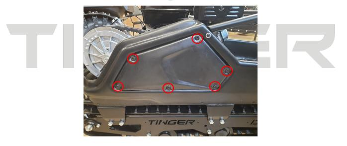
6. Unscrew the bolts that are anchoring the underframe with the reverse gearbox to the frame.
