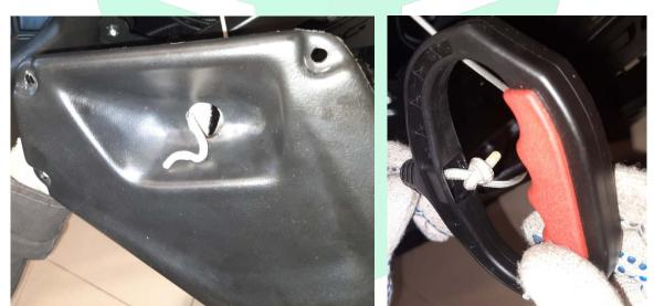
45. Take the tool out of the loop and untie the loop. Holding the side cap and handle, return the cable back to the place.
