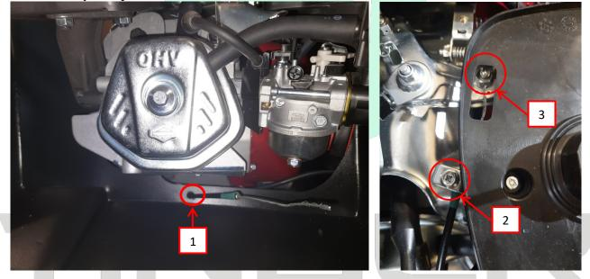
33. Take the M7 cable tensioner bolt and 3mm cable fixator and  $\emptyset$ 14 mm spring out of the «Spirings and retainers kit» package No6. Connect the throttle choke cable with yellow braid.
