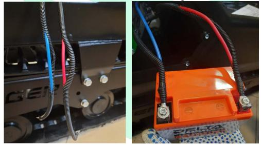
41. Install the accumulation battery at the engine compartment behind the CVT. Take the accumulation battery fastener belt out of the package  $N_{2}7$ . Anchor the fastener belt with a tongue to the hook behind the accumulation battery. Anchor the belt hook at the front of the battery to the hook by tightening the the belt tongue.
