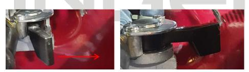
2. Press the brake handle till stop and set the red handbrake to the right.
