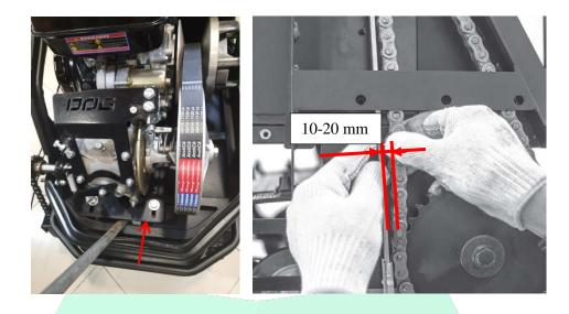
31. Tighten bolts that fasten underframe to the frame of the towing sled.
