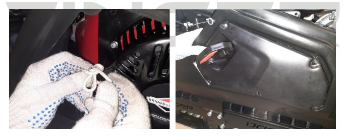
46. Fix the side cap, using the screws with inner hex.
