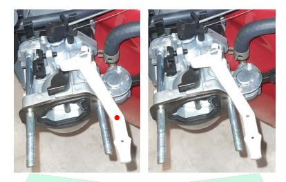
18. Install the manifold at the original place, anchor it by bolts. Connect the hose.
