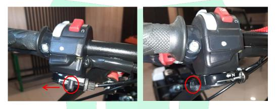
4. Apply power to the engine –move apply power switcher on the handlebar switch to the lower position.
