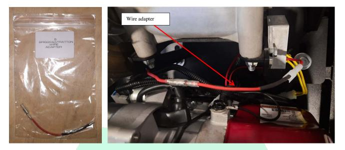
39. Connect wires to the accumulation battery terminals by the given way: the red wire in the corrugation to the «+» terminal. Connect the blue wire in the corrugation to the «-» terminal.
